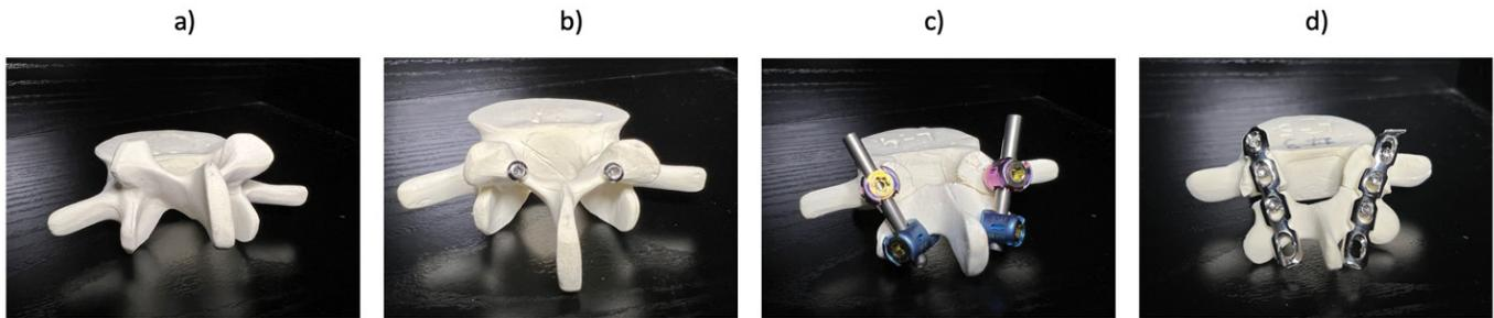
**Figure 1:** Intact (a) and Fractured Sawbones with fixations for pars fractures: b) Bucks' Screw Model, c) Pedicle Screw Laminar Hook Model, d) Pars Interarticularis Plating Model
