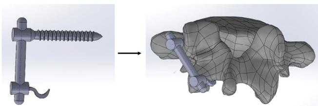
**Figure 5:** FEA Models of Hook-Screw and insertion into fractured vertebral model
