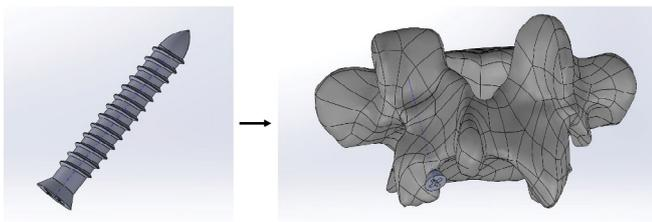
**Figure 4:** FEA Models of Buck's Screw and insertion into fractured vertebral model
