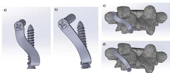
**Figure 6:** FEA models of the novel design paradigms conceptualized by the Biomechanical Research Laboratory. a&c) Implant 1, b&d) Implant 2
