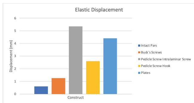
Figure 8: Elastic Displacement Results
