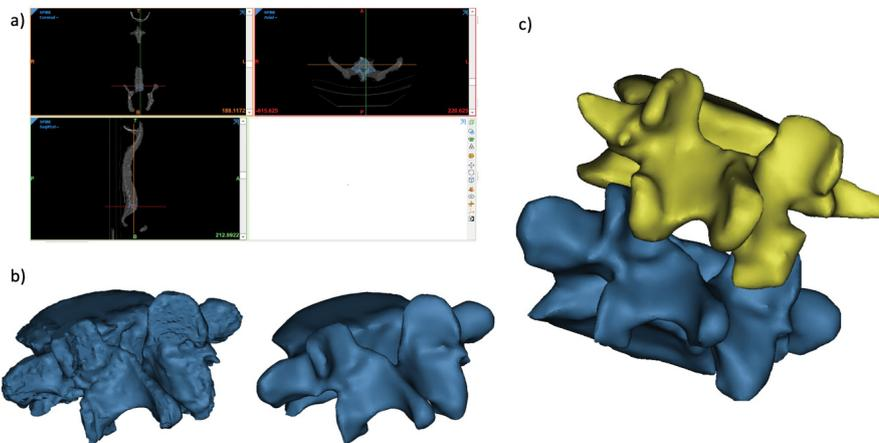
**Figure 3:** L4-L5 vertebrae modeling. a) Mimics view, b) L5 vertebra model in Mimics before and after smoothing and wrapping operation, c) L4-L5 final vertebra model
