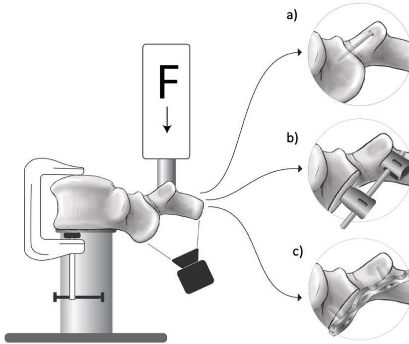
**Figure 2:** Diagram of SawBone Testing Frame. a) Bucks Screw Model, b) Pedicle Screw Laminar Hook Model, c) Pars Interarticularis Plating Model
